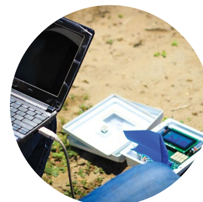
Pictured is the computer connected to the soil sensors to collect and store moisture readings directly from the field. The information will be used to make an informed irrigation decision.
